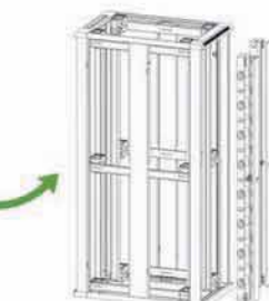
2B. Assemble frame, cable management slot(only width 800mm). (screw M5x10).
